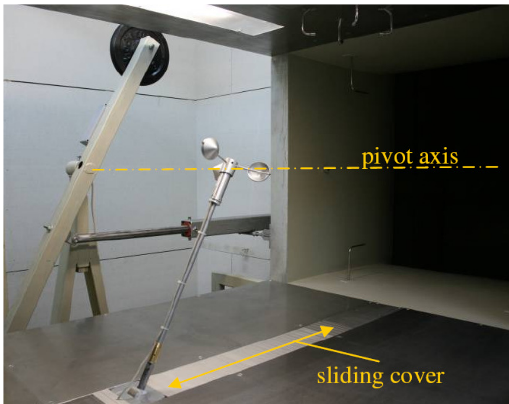
Figure 15 Tilting mechanism of WT II with sliding cover
