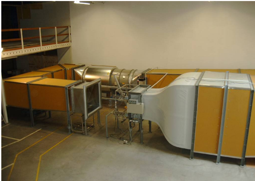
Figure 2: Wind tunnel I of Deutsche WindGuard Wind Tunnel Services GmbH used for anemometer calibration and testing (picture dated 2005)
