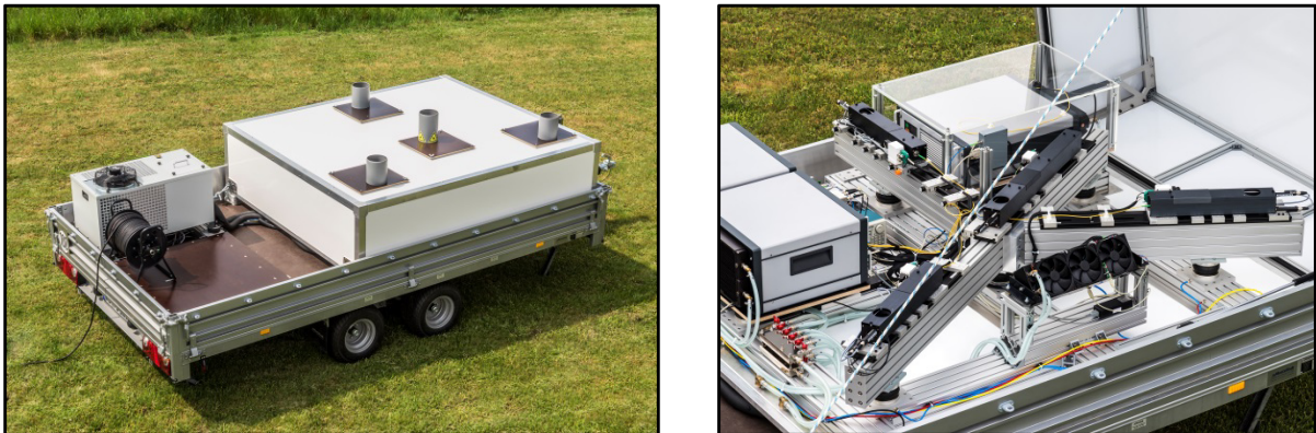
Figure 4: PTB trailer with the prototype of the bistatic Lidar and view onto the set-up inside the housing
