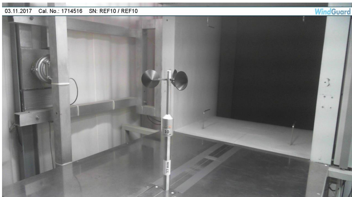
Figure 1: Setup of the SQC anemometer 'REF10', type 4.3351.xx.xxx in wind tunnel 'Varel 1'.
