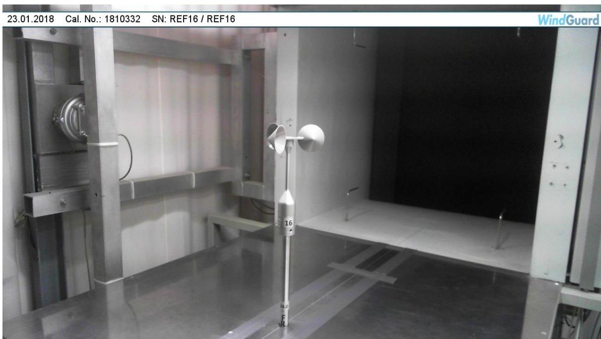
Figure 1: Setup of the SQC anemometer 'REF16', type P2546A-OPR in wind tunnel 'Varel 1'.
