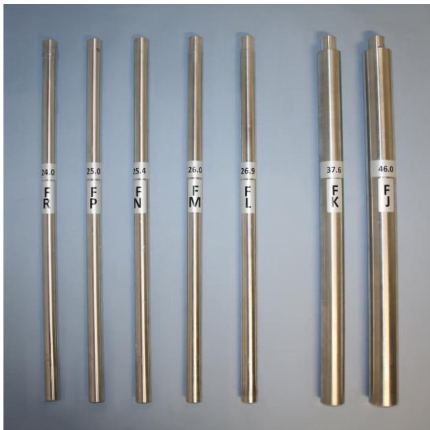
Figure 4: Seven mounting pipes with different diameters manufactured for the tests with the WindSensor and Windspeed anemometer.
