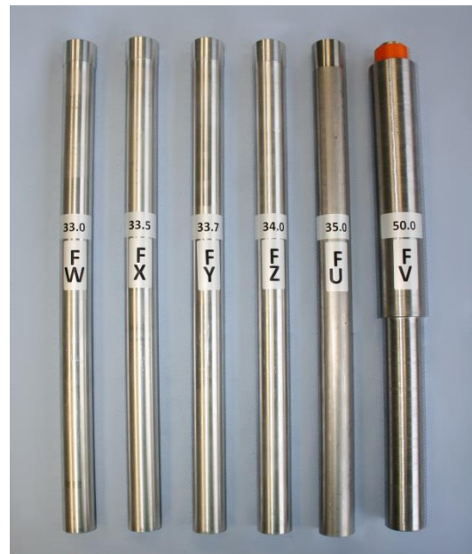
Figure 5: Seven mounting pipes with different diameters partially supplied by Thies. FU is a customized mounting tube supplied by DTU.
