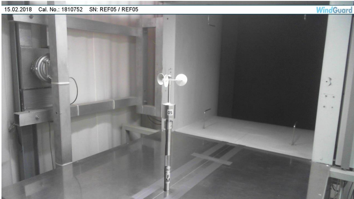
Figure 2: Setup of the SQC anemometer 'REF05', type A100L2 in wind tunnel 'Varel 1'. Remark: The proportions of the set-up may not be true to scale due to imaging geometry.
